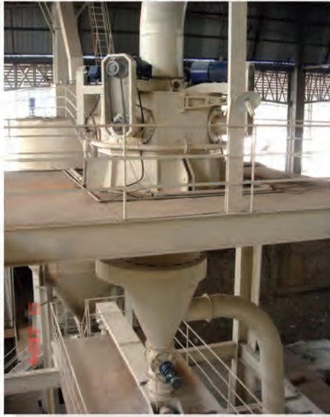
图为加工组装完毕的超细分级机 The picture shows completed assembly of Super Fine Classifier
