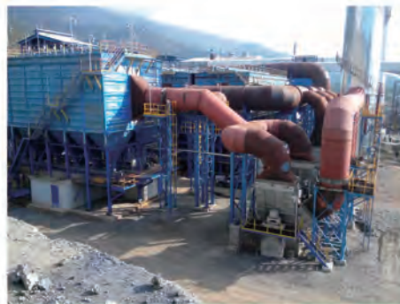
Large-scale High-temperature Bag Filter for Steel Plants used at Guatemala Steel Plant
