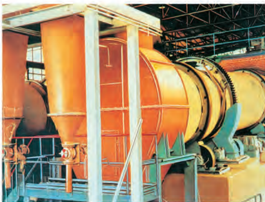
用于江苏龙潭水泥厂3x20m矿渣烘干系统 New Type Energy-saving Rotary Dryer used at Jiangsu Longtan Cement Plant
