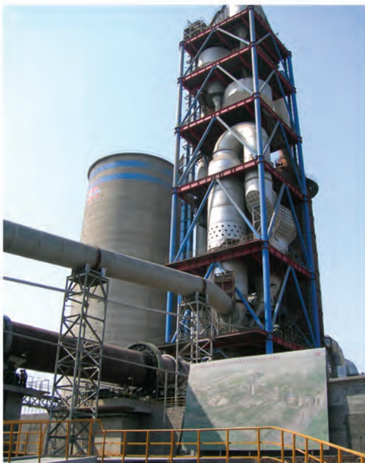
郴州东江金磊水泥有限责任公司2500t/d熟料生产线 Hunan Jinlei Cement Corporation 2500t/d clinker production line
