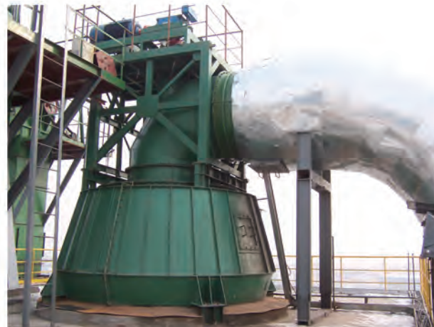
自主研发的高效选粉机 High Efficiency Separator developed by HCRDI
