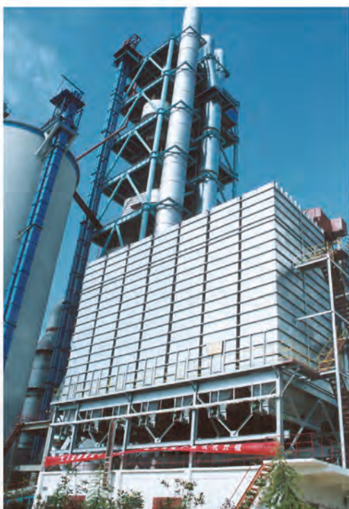
南阳航天水泥厂6000t/d 熟料生产线窑尾高温玻纤袋收尘器 High Temperature Glass Fabric Dust Collector used on kiln inlet at Nanyang Cement Plant
