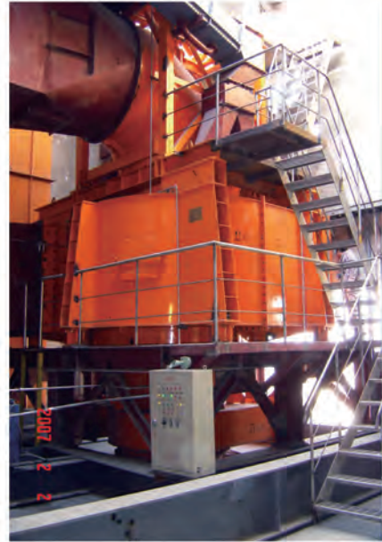
自主研发的高效选粉机 High Efficiency Separator developed by HCRDI
