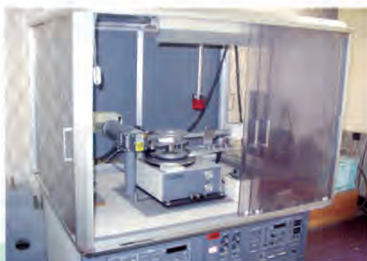
大型精密仪器——X射线衍射仪，可对物相进行精确测定 X-ray diffraction analyser is now making accurate measurement for substantial phase of the material
